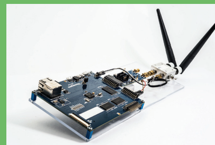
IMEC and Analog Devices' prototype low-power highly accurate indoor localisation sensor
