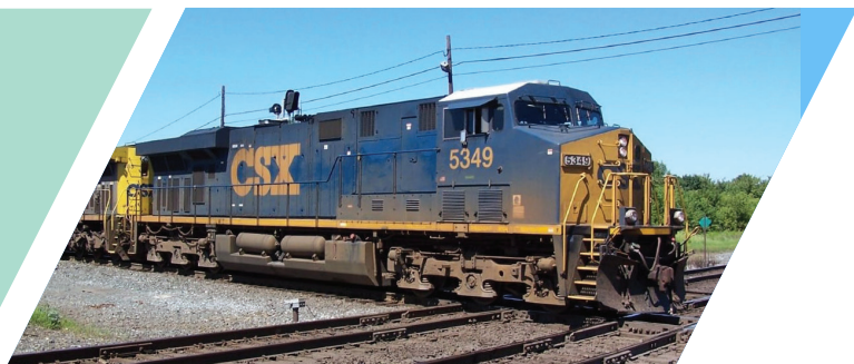
Figure 1: The General Electric ES44DC Locomotive is a fully-automated industrial diesel powerplant on wheels, generating 4,400 hp (3,280 kW). It's 250 sensors continuously monitor the engine and environment to automatically control throttle and brakes. (source: Wikipedia)
