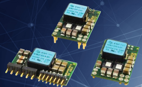
Figure 4: This all-digital DC/DC PoL converter from CUI delivers up to 50A and is part of a family of both larger and smaller efficient, flexible, compatible and feature-rich DC/DC converters for larger application needs. (Image: CUI Inc.)
