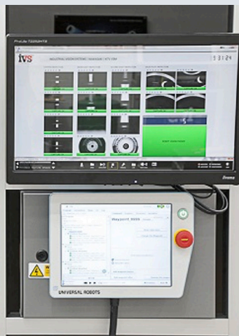
A cobot equipped with a MVS for quality inspection. Image credit: Kawasaki Precision Machinery and Industrial Vision UK
