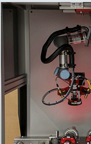
A cobot equipped with a MVS for quality inspection. Image credit: Kawasaki Precision Machinery and Industrial Vision UK
