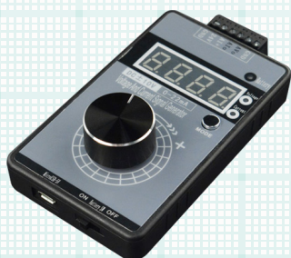
Figure 3: A single rotary-push knob makes for easy configuration of the DFRobot FIT0778 handheld signal generator.
