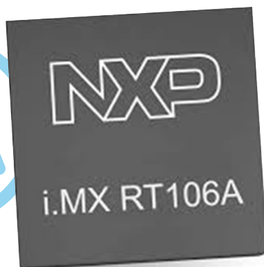
Figure 3: NXP Semiconductors i.MX RT106A Crossover Processor. (Source: Mouser Electronics)
