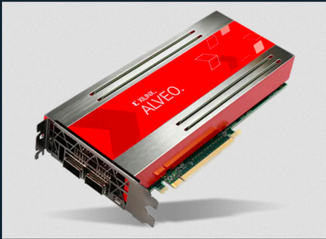
Figure 2: Xilinx Alveo Accelerator card (Source: Mouser Electronics)
